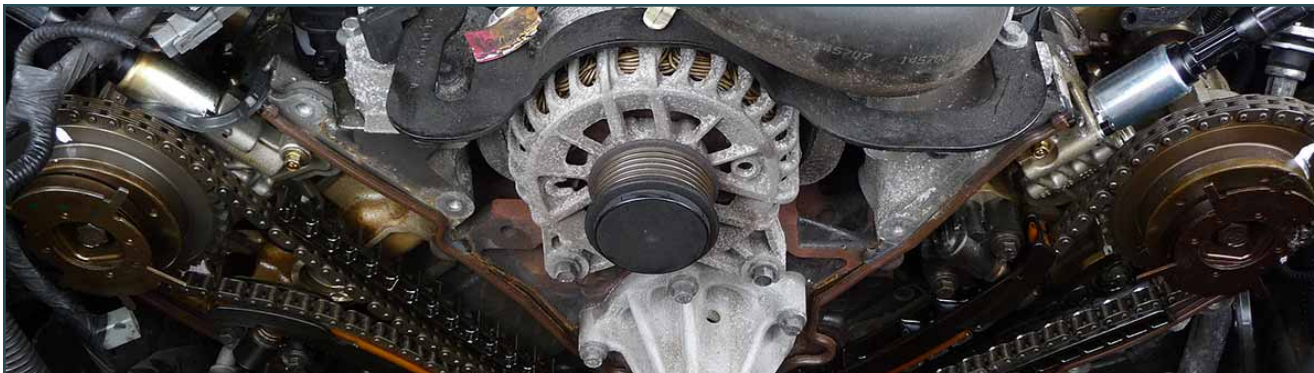
Figure 7: The crank lined up so the keyway was up at the 12 o'clock position.
