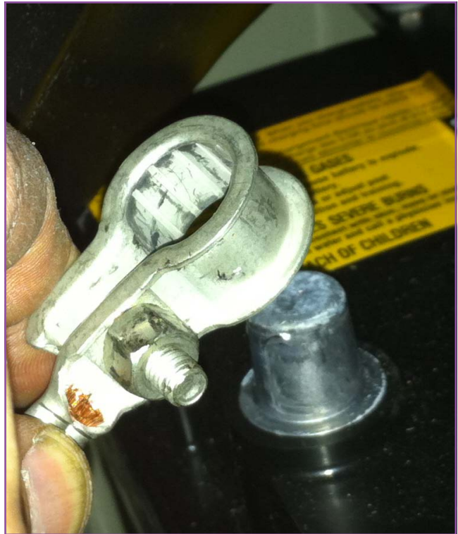
First disconnect the 12V battery. This will prevent a myriad of potential problems.
