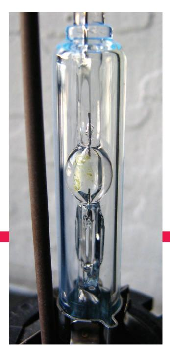
There's no dirt in this bulb! You can see the metal compound in its solid state up close.
