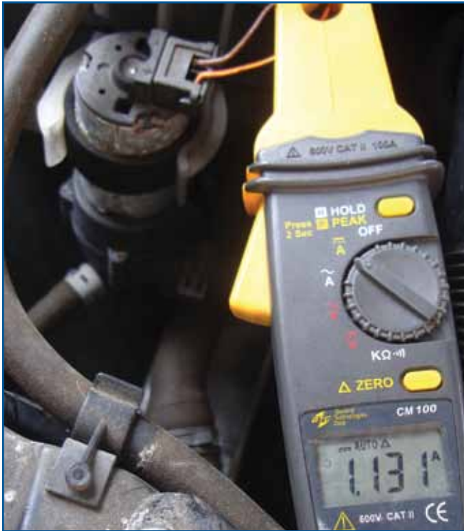
Newer auxiliary coolant pumps have good accessibility. You can easily measure the amp draw while you set the controls to maximum heat. This reading of over one amp is good.
