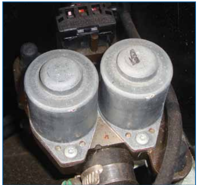
If the duo-valve is accessible, you can check the electrical signals on the two outside pins of the three-pin connector. This C43 has power on the center pin, and the two outer pins are grounded to close the valve.
