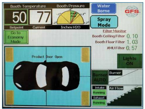
A modern paint booth has settings to optimize the treatment of water-based paints. The unit is programmed to control each step of the refinishing process and is a worthwhile investment for higher-volume facilities.
