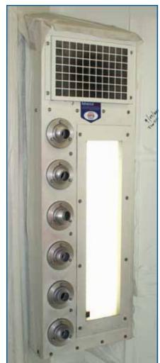
Remember, temperature is not as much of a factor in drying waterborne paints as increased airflow, which will reduce your flash-off time between coats.
