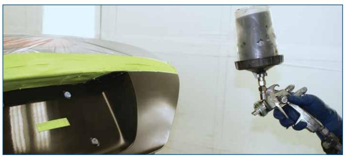
You should be aiming for a one mil coat when spraying a panel. This should take one to one and a half applications if done properly. You should apply around 30 psi to your gun until you get a feel for the technique.
