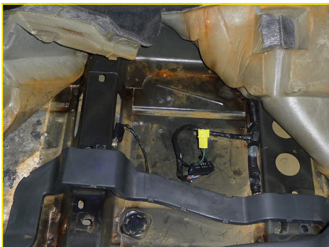
Figure 5: Lifting the rug, noticing a lot of rust build-up on the floor from a prior water leak.
