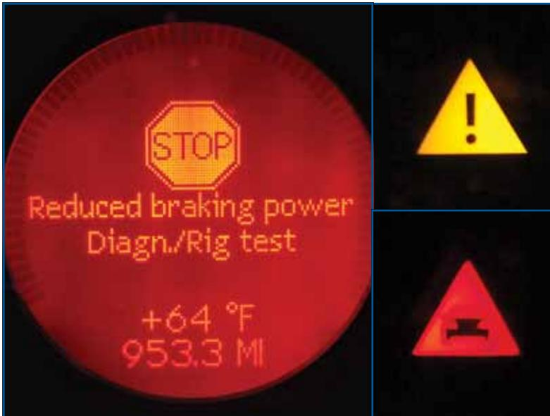
When the SBC is deactivated, or there is a failure in the system, you will see a warning message in the instrument cluster. Pull codes and look at pressure in the system before disconnecting any brake lines.
