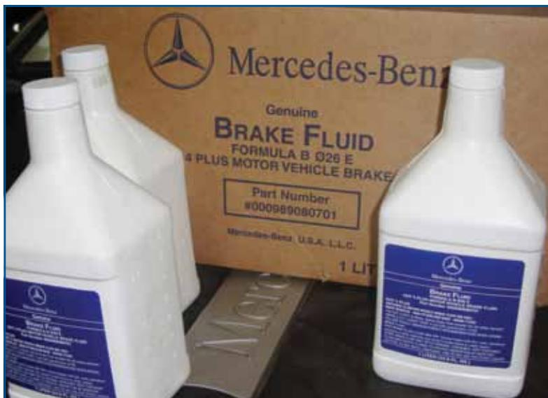
*While picking up SBC components at your Mercedes-Benz dealer, you should purchase at least two liters of approved brake fluid to completely bleed the system. Since brake fluid is hygroscopic, it is recommended that it be replaced every two years as normal maintenance.*
