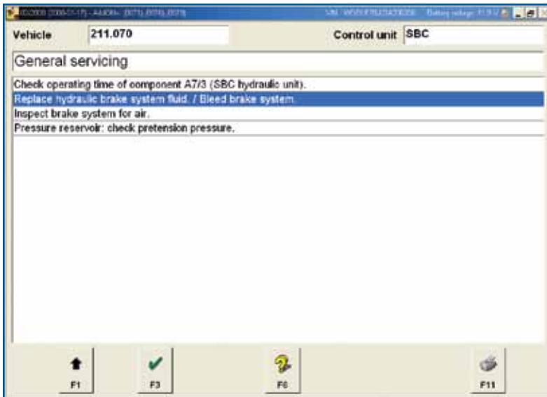
Follow the steps outlined in the bleed procedure in your SDS unit. Make sure to secure your brake bleeder lines to the screws since high pressure brake fluid comes out when opened.
