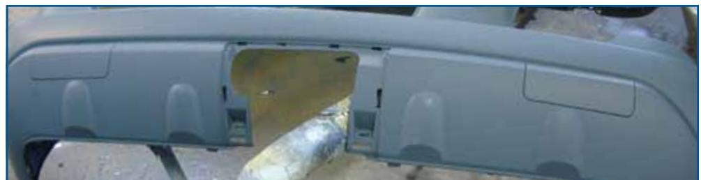
Even with light hits, using OEM parts like this ML rear bumper cover will reduce labor time. You will not have to modify the part to make it fit. It comes already primed so all you have to do is prep it for painting.
