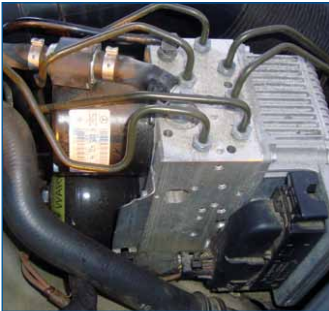
The heart of the Sensotronic braking is the SBC hydraulic unit. You can see the high-pressure hydraulic pump on the left and a pressure reservoir below it. This unit actually produces the fluid psi that stops the vehicle.
