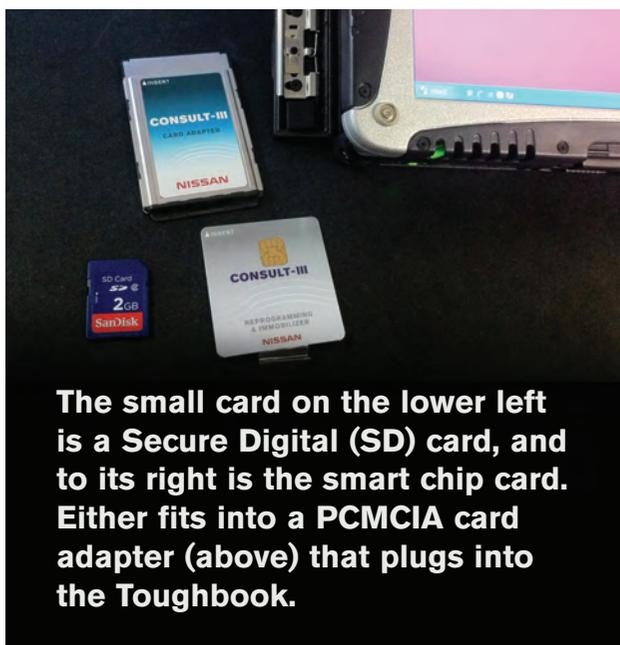
**The small card on the lower left is a Secure Digital (SD) card, and to its right is the smart chip card. Either fits into a PCMCIA card adapter (above) that plugs into the Toughbook.**
