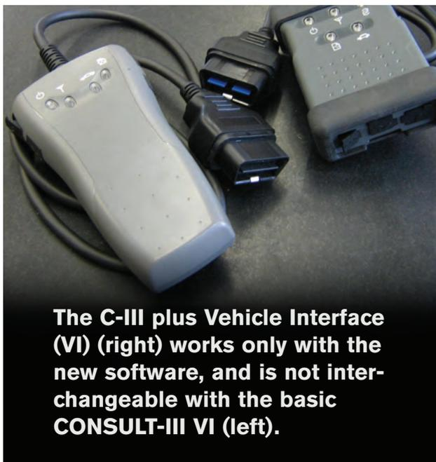
**The C-III plus Vehicle Interface (VI) (right) works only with the new software, and is not interchangeable with the basic CONSULT-III VI (left).**
