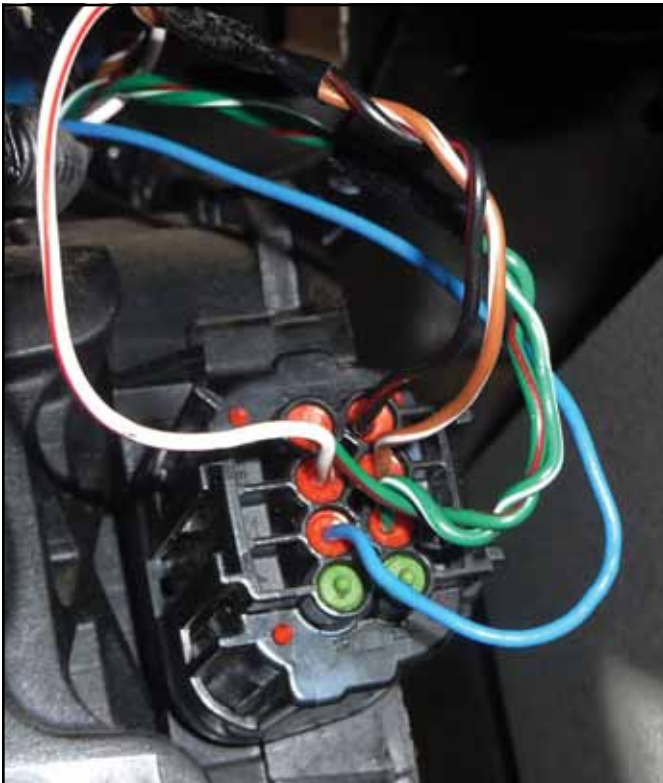
Figure 3: APP Sensor located at gas pedal.
