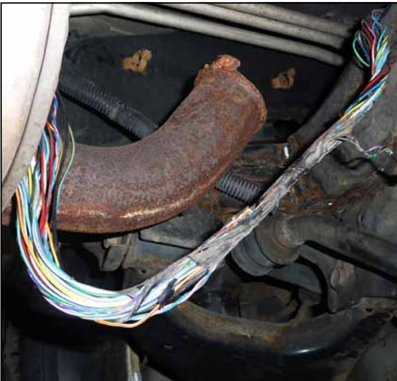
Figure 12: Melted ECM harness at R/R suspension from broken tailpipe.
