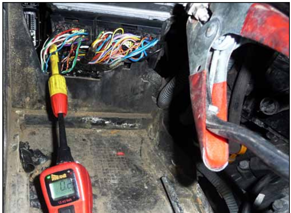
Figure 6: APP Sensor #1 Ref Voltage reading at ECM.
