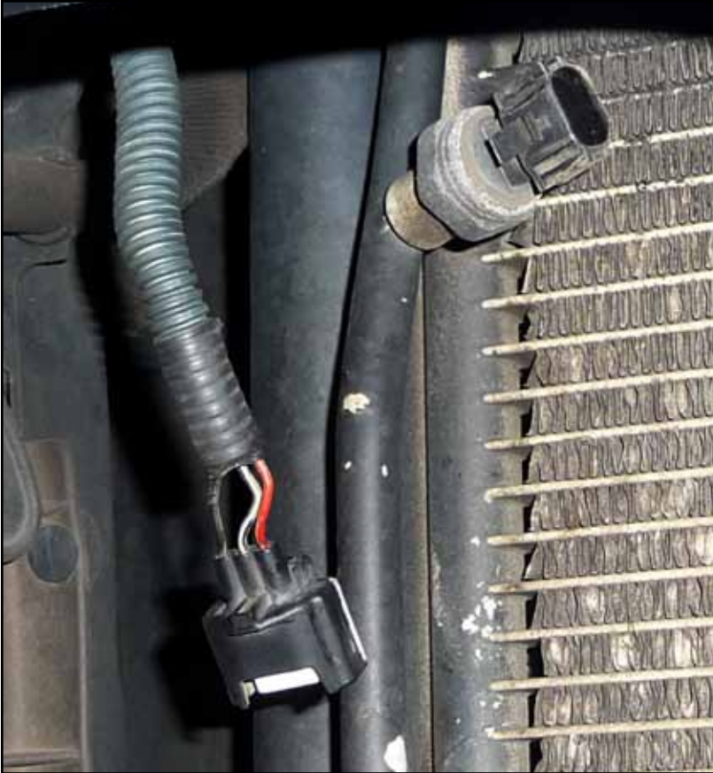
Figure 11: A/C Pressure Switch unplugged.
