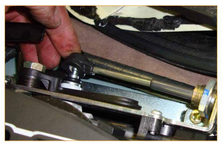
Here is the important adjustment of the shifter cable. With the lever on the transmission and the shifter both in Park, put the ball in the socket. Then, pull on the cable housing lightly and tighten the locknuts on the bracket. As you move the shifter, the trans lever should move with it.
