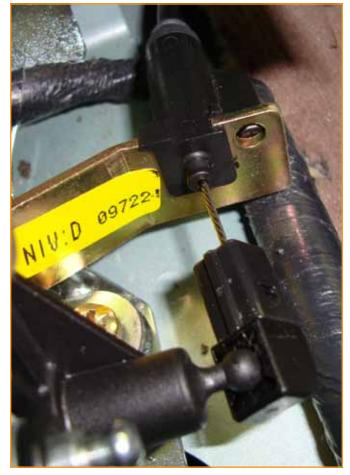
Don't forget to attach the key interlock cable. This isn't adjustable, but it doesn't need to be to get the key out of the ignition switch. While it's disconnected, pull on the cable and make sure it doesn't stick.
