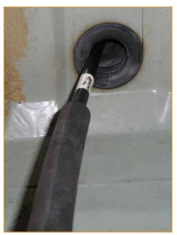
Fish the shift cable through the hole in the floor. Be careful not to twist it into an unusual position or it might bind. Fully seat the grommet in the hole to keep moisture out (it also keeps the cable housing from flexing).
