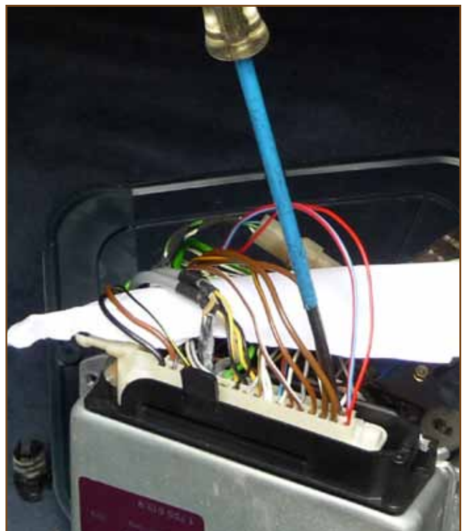
Figure 5: Checking for ECM power feed
