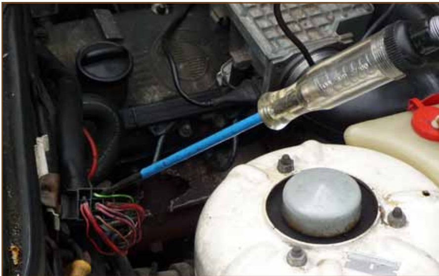
Figure 7: Checking ECM relay coil feed
