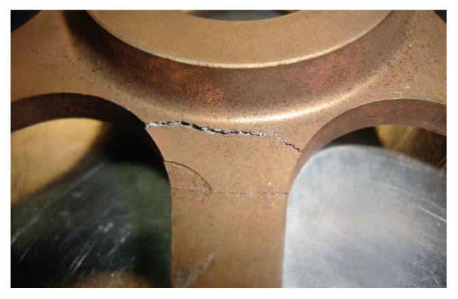
These cam sprockets need to be on tight. If you try to remove one with a standard puller, you may damage it. Inspect the sprocket for cracks, such as this one has.
