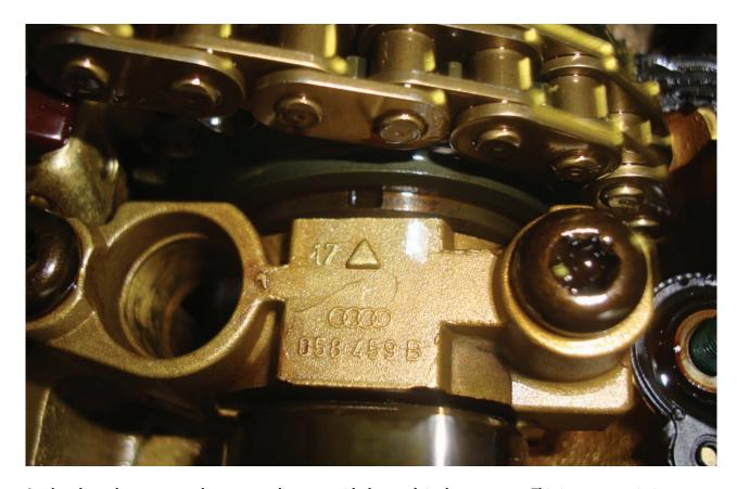
Look at how the arrow on the cam cap lines up with the notch in the cam gear. This is a correct timing setup. The white paint mark you see was where the notch was lined up. The intake cam had to be moved to the left one tooth on the sprocket.
