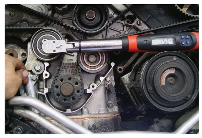
Notice how we are preloading the tensioner to 15Nm of torque. This pulls the belt tight around all the sprockets and pulleys. At this point we can pull the pin to release the tensioner. The next step is to tighten the cam gear bolts to 55Nm to secure them.
