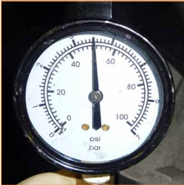
Figure 5: At idle, with foot off the brake pedal, pressure was within specifications at about 50psi.
