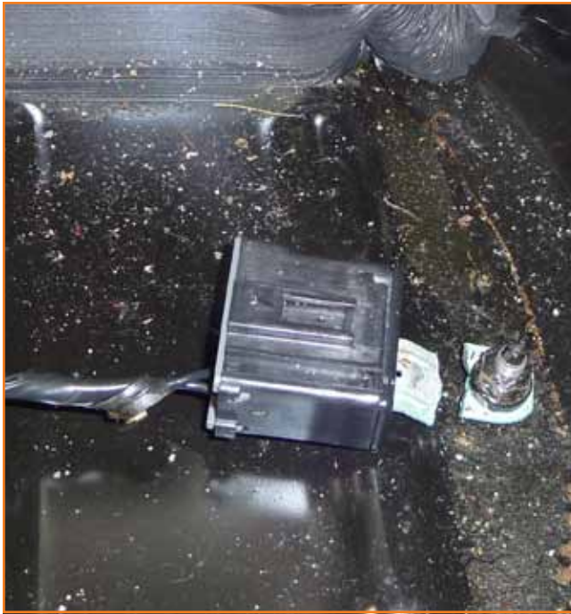
Figure 9: Broken ground found in the right rear cargo compartment.
