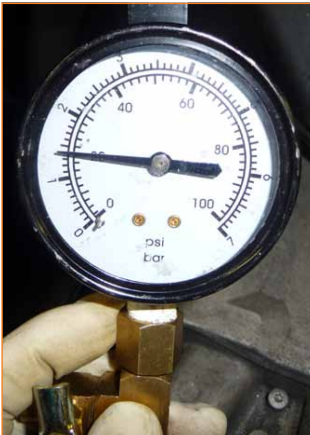
Figure 6: Applying the brake pedal, pressure dropped to about 20psi.
