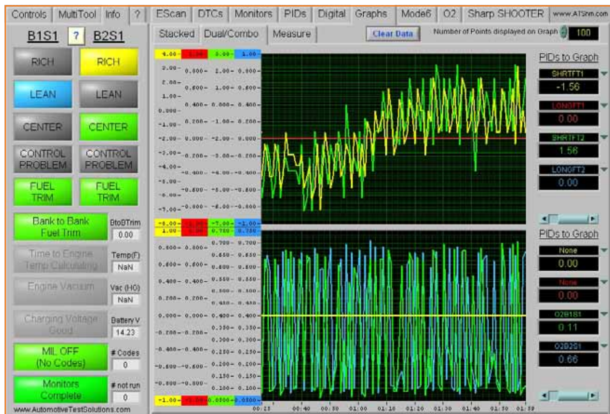
Figure 3 (Above): O2 sensors and fuel trims with the engine idling and all seem okay. Figure 4 (Below): Stepping on the brake pedal, both O2 sensors went lean & the short-term fuel trim maximized to positive 25% without the PCM achieving any fuel control.
