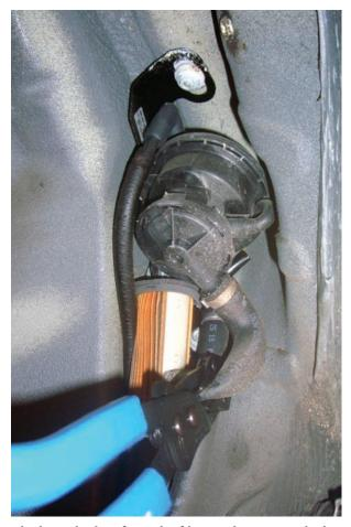
Blocking the line from the filter to the LDP seals the system. Any smoke you see must be coming from a leak. If there are no leaks, the ball in the flow meter should drop completely.
