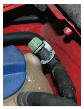
If you have the proper fitting, you can pipe directly into the test port and add smoke. If you do not have this fitting, you can add smoke to the canister side of the canister purge solenoid. It may time out a few times before you get enough smoke into the tank.
