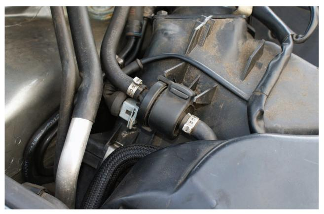
The Canister Purge solenoid is usually located on the passenger's side inner fender. You can inject smoke here if you need to. You can also remove the canister line and listen for a pulsing vacuum sound. If the sound is steady, the solenoid is stuck open. You will also get a P0171/4 from the lean condition at idle.
