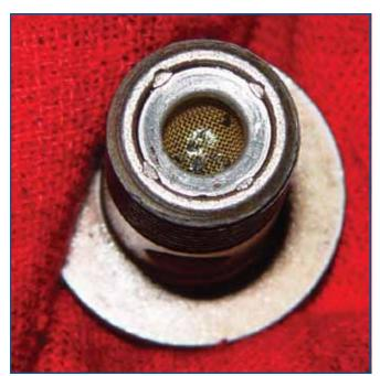
You'll find a screen in the banjo bolt of the pressure feed line. It protects the system by blocking debris. It should be removed and cleaned whenever service work is done to prevent pressure drop in the system.
