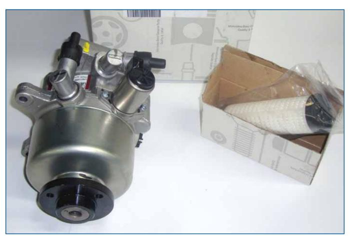
The return-flow filter is mounted in the reservoir. While you're visiting your Mercedes-Benz parts dealer, you should pick up these filters and at least four liters of hydraulic fluid. This will protect your work and give components the longest possible service life.
