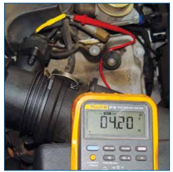
With a quality DMM (Digital Multi-Meter) you can measure signal voltage using the MAX/MIN feature. While recording, accelerate to WOT and see what your maximum voltage is. A good MAF should read over 4.0V. If not, you probably have a fuel trim code with high Multiplicative readings.
