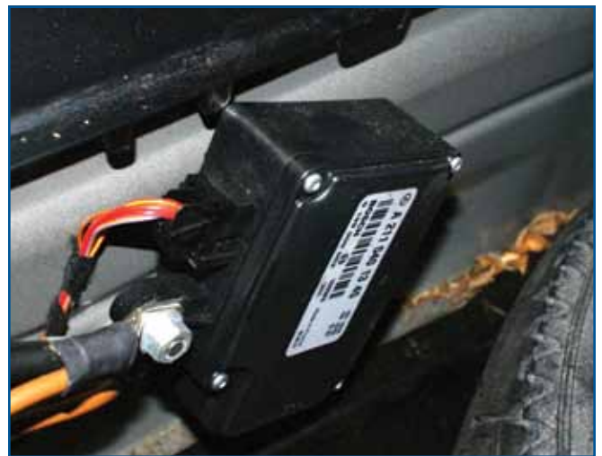
The battery control module, pictured here, monitors the rear battery voltage, the front battery voltage, and alternator output through the body CAN B. You can talk to it with your SDS unit and program it if it needs to be replaced.
