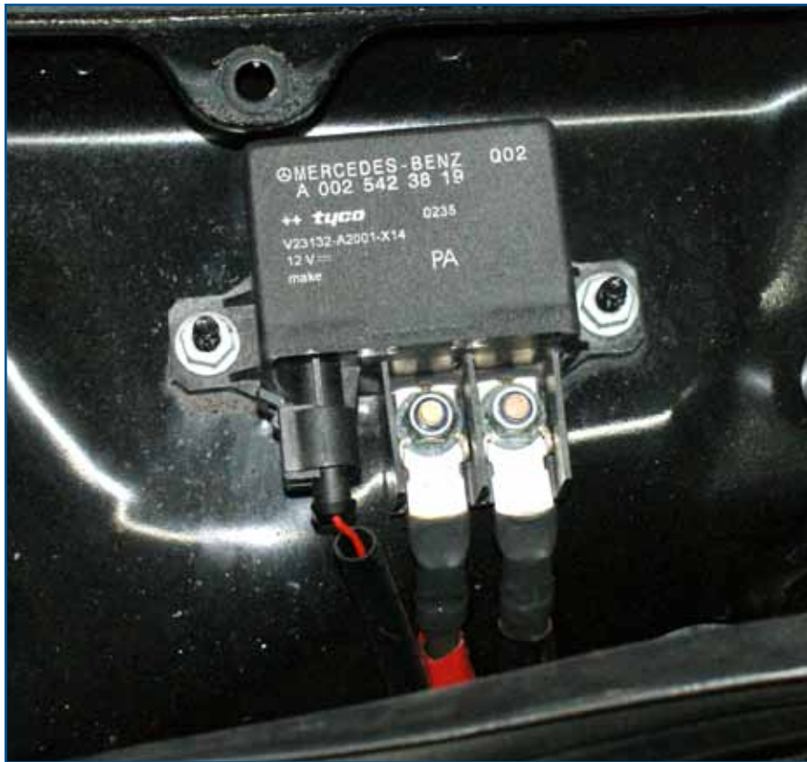
This is the auxiliary battery relay. It turns on to allow the auxiliary battery to charge and, if system voltage is low, to add current under heavier loads. It is not on all the time, so do not expect the auxiliary battery to always indicate charging voltage.
