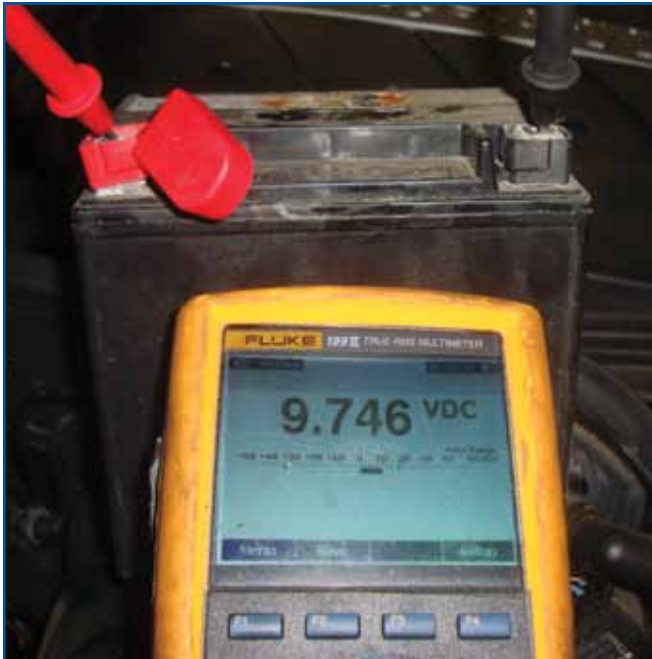
This auxiliary battery has seen better days. It should supply 12.6 to 12.8 volts when properly charged. This one can no longer hold a charge. The black case tells you to check if it is an AGM type. In this case, it is. Using an OEM battery is the safest way to repair the problem and prevent false alarms in the future.
