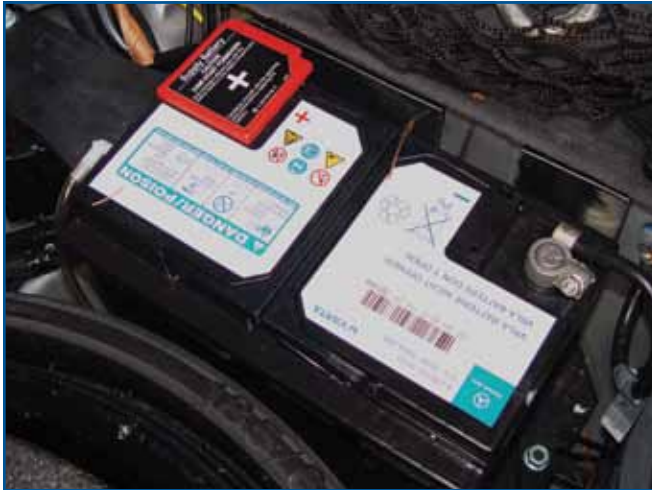
This rear-mounted battery is the main electrical power supply in some newer systems. A black case tells you it is an AGM battery. Read the warning on the red cover and look for the letters "VRLA" to confirm. You'll need a special battery tester to check this one.
