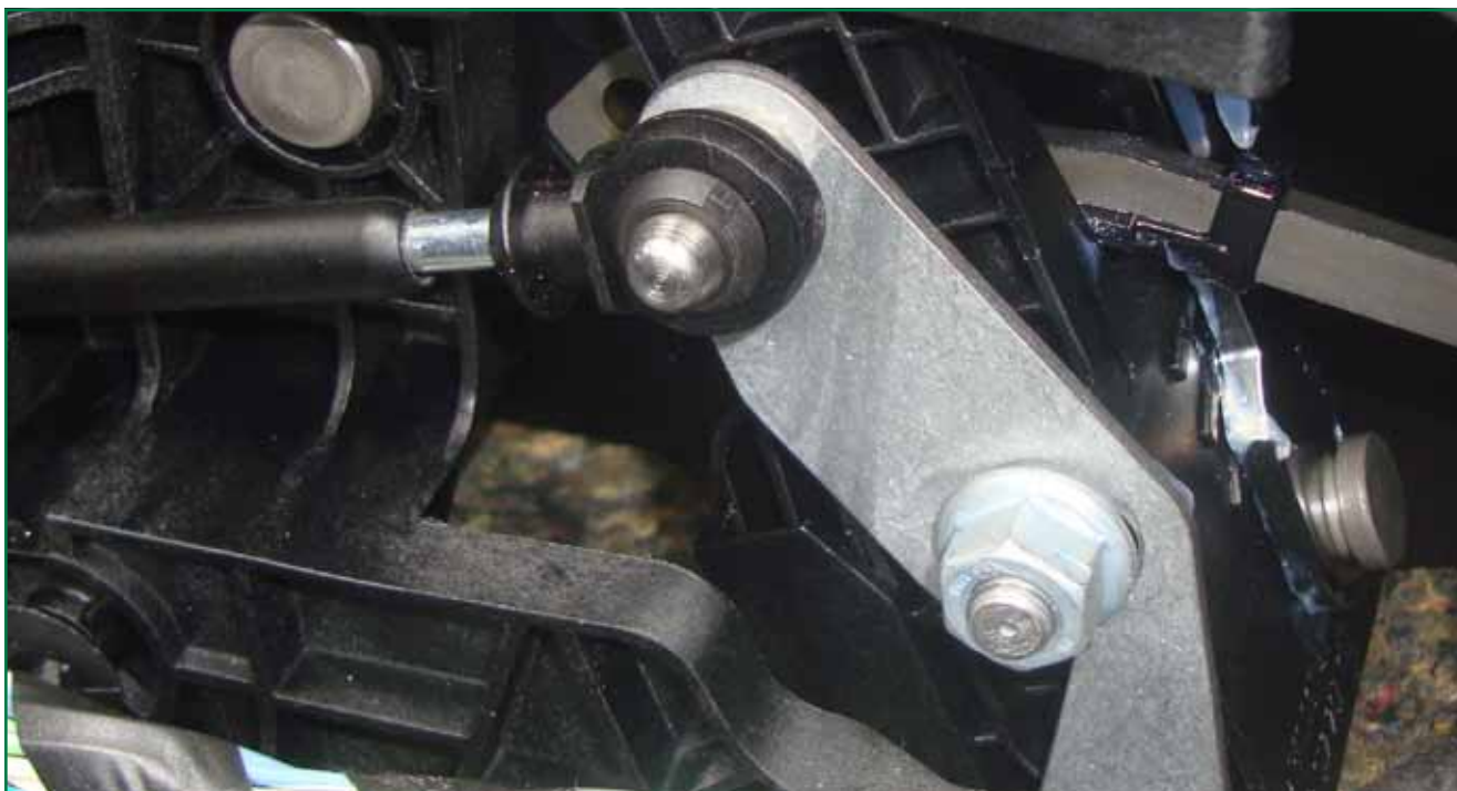
When installing the shifter, put it in park. Pull on the shift cable all the way rearward, then position the lever so you can pop the ball socket on the lever. Then tighten the 13mm nut to secure the adjustment.
