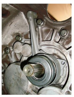
Newer manual gearboxes have the slave cylinder and throw-out bearing as one piece mounted inside the transmission bell-housing. This unit should be replaced while servicing the clutch. Special bleeding procedures are required, so go to www.erwin.vw.com for specific technical information.
