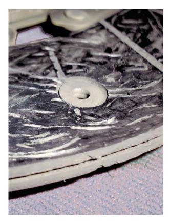
Look at the rivet head on this clutch disc. The flywheel side of the fiber plate is just about worn down to it. Luckily, the rivet is not gouging into the flywheel. This disc needs to be replaced.
