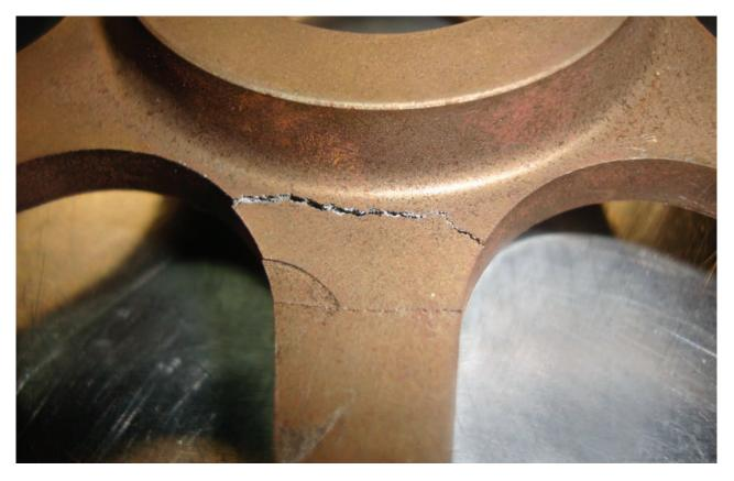
These cam sprockets need to be on tight. If you try to remove one with a standard puller, you may damage it. Inspect the sprocket for cracks, such as this one has.
