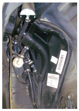
To capture vapors during refueling, Volkswagen vehicles have an expansion tank as part of the filler neck. This holds fuel vapors, separates liquid fuel and returns it back to the fuel tank. You may have to add smoke from the gas cap if you suspect a leak here.
