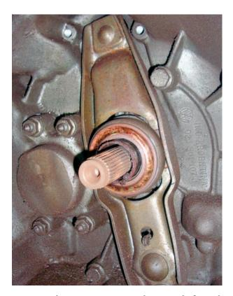
Here we have a conventional input shaft and throw-out bearing. Before installing, clean the splines and shaft as well as possible and lubricate with wheel bearing grease. Anti-seize compound is a poor lubricant, and tends to fling off onto the friction material.
