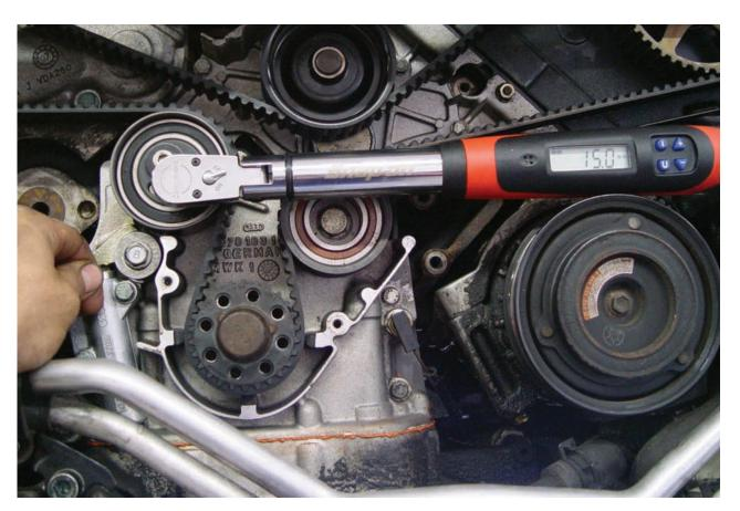
Notice how we are preloading the tensioner to 15Nm of torque. This pulls the belt tight around all the sprockets and pulleys. At this point we can pull the pin to release the tensioner. The next step is to tighten the cam gear bolts to 55Nm to secure them.
