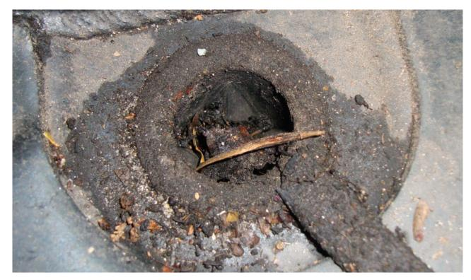
Make sure the cowl drains are not clogged, which would allow standing water to migrate into the body. This can build up underneath the carpeting without the customer even knowing. On Passat models, this means removing the battery for access.
