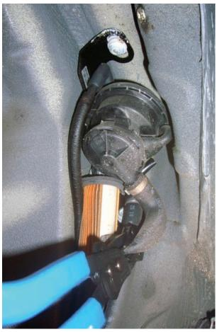
Blocking the line from the filter to the LDP seals the system. Any smoke you see must be coming from a leak. If there are no leaks, the ball in the flow meter should drop completely.
