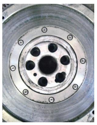
Is that flywheel worth machining? If you remove any material from the inside friction surface, you will also need to machine the outer step. This means pins need to be pulled and reinserted.
