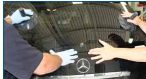
Set the glass properly the first time. Today's quick-curing sealers don't allow much forgiveness.
