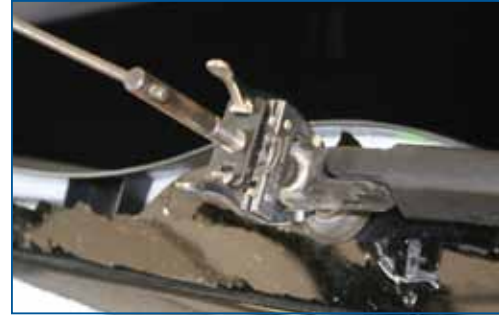
To avoid costly damage, take care when removing the wiper arm.
