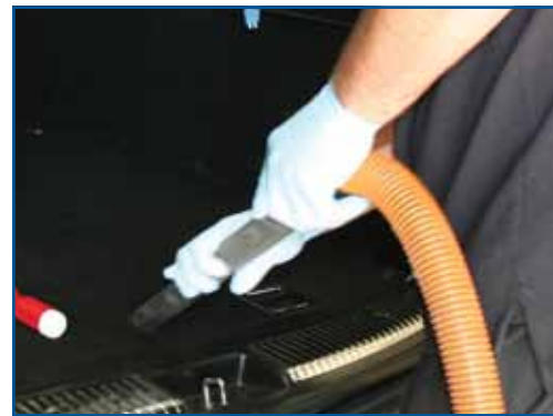
Be sure to remove all glass shards and particles from the vehicle to avoid angering the customer.
