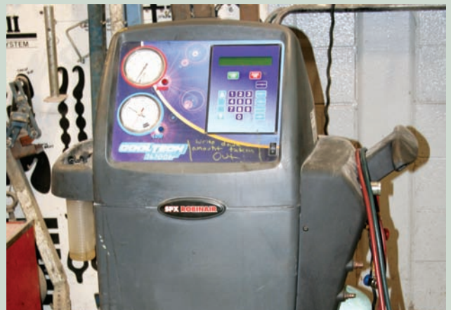
An R134 refrigerant recharging/recovery/recycling station helps you meet regulations, saves time and holds down costs.
