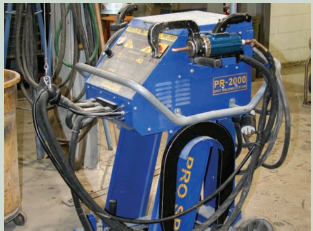
A spot welder and an assortment of tips ensures the strongest welds.
