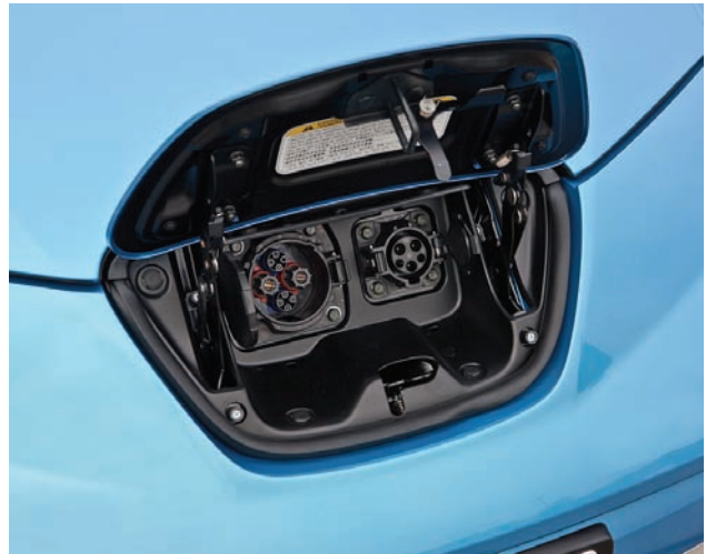
The Leaf 220/240V Level 2 (right) and 440/480V Level 3 (left) charging ports are located under a panel above the front bumper.
