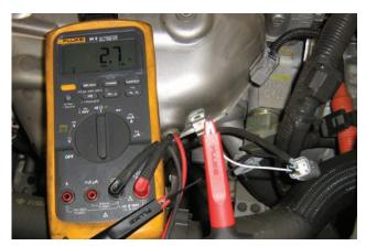
Check the heater element resistance with an ohmmeter.
