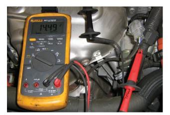
Check for power while the heater is operating.
