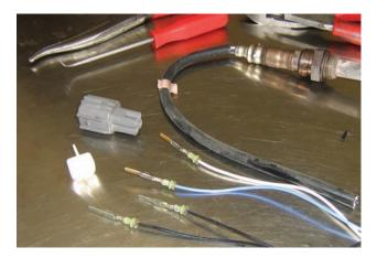
TIP: Disassemble and scavenge terminals from the O2 and A/F sensor sensors you replace. Some are male and some are female. They come in handy to make a solid DMM connection for future testing.
