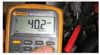
An oscilloscope will provide more information, but a DMM that can measure Hz, duty cycle, or pulse width can also be used for a quick check of ECM heater control.
