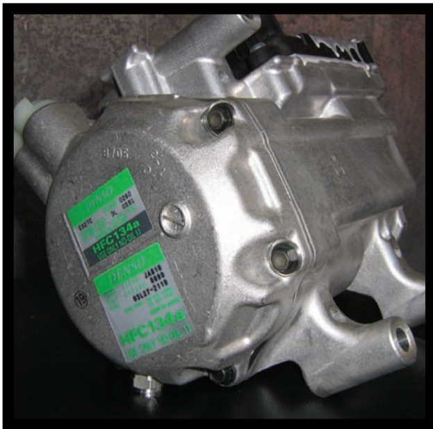
The Altima hybrid's electric compressor has a sticker indicating the required refrigerant R134a and special oil, ND-OIL 11.
