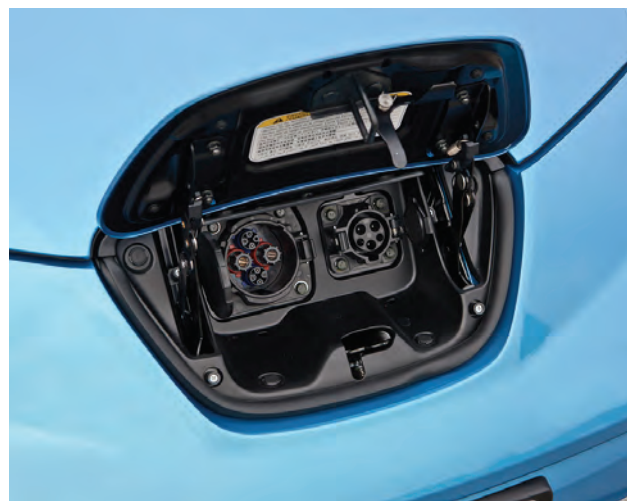
The Leaf 220/240V Level 2 (right) and 440/480V Level 3 (left) charging ports are located under a panel above the front bumper.
