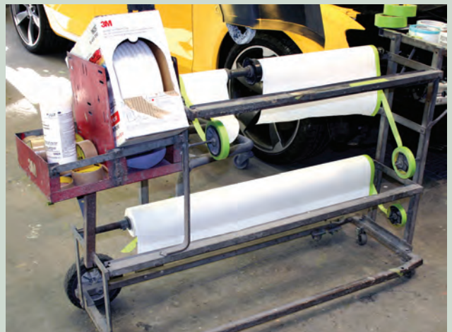
A masking paper and tape dispenser saves time and gets the job done right.
