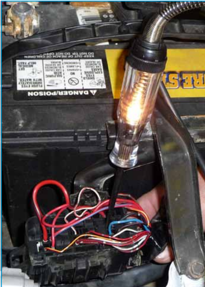
Figure 8: Back probing the O2 heater relay to check contact feed to O2 heaters.
