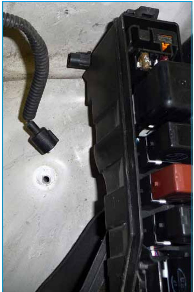
Figure 10: Open O2 heater circuit under the battery tray.
