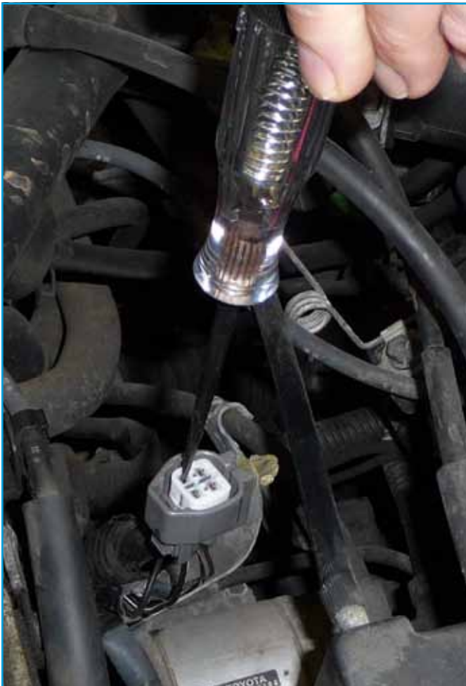
Figure 9: Testing the B2S1 O2 heater connector for power supply.
