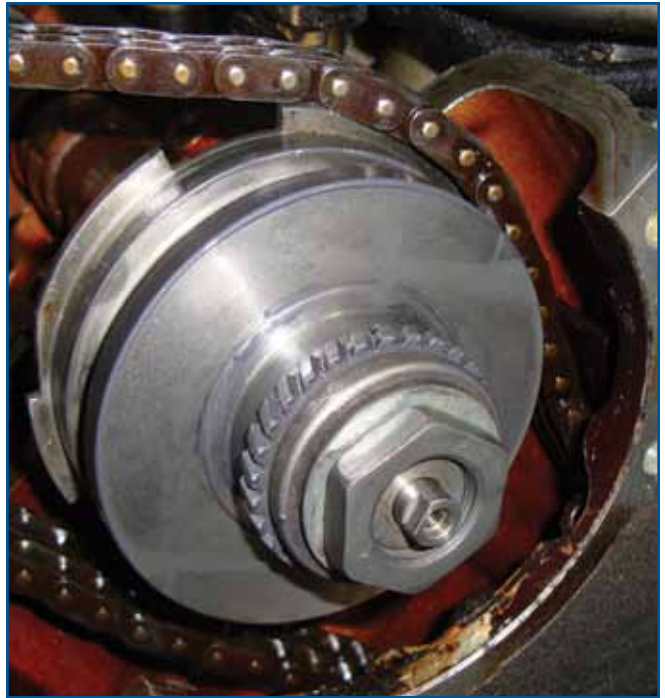
First, you attach the cam adjuster inner plate to the mount with new bolts. Then, install the spring. You could use the old nut to temporarily hold the assembly together while you add the outer cam sprocket.
