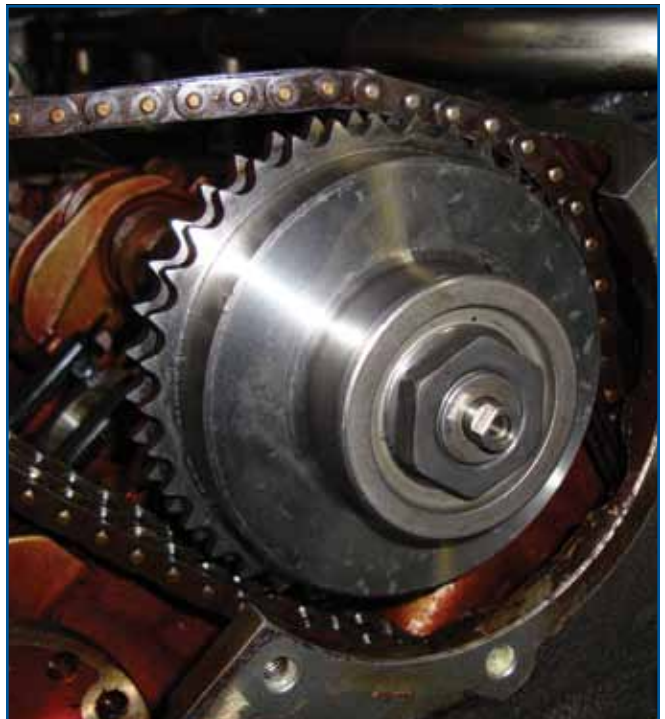
Hold the assembly together and remove the camshaft adjuster mounting nut. Then, install the new nut with the large washer that holds the assembly together. This nut must have the proper torque applied to it, which you can get from WIS in Startekinfo.
