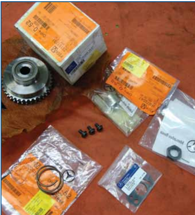
When changing the camshaft adjuster unit, you should also replace the return spring. You will also need to get new mounting hardware and properly torque it down so there will be no issues in the future. Since you had to remove the tensioner, you should include a new gasket.
