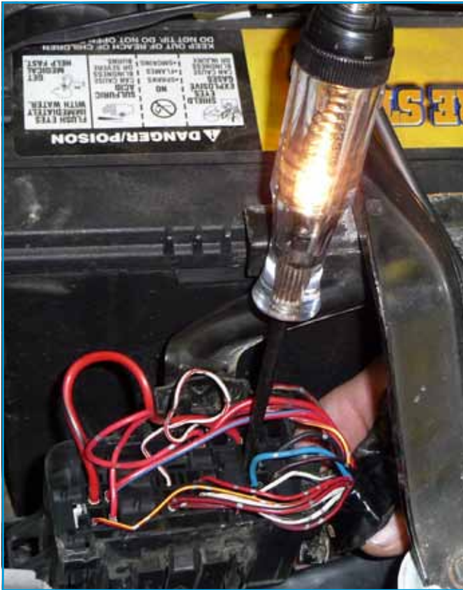
Figure 8: Back probing the O2 heater relay to check contact feed to O2 heaters.
