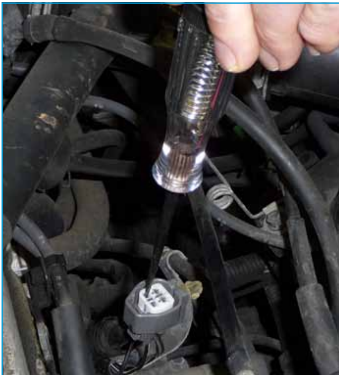
Figure 9: Testing the B2S1 O2 heater connector for power supply.
