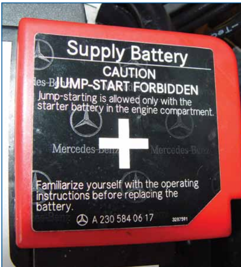
Don't discard the systems battery's positive post cover as it carries the warning not to jump start the vehicle from this post. Also, these VRLA/AGM batteries should not be charged as you would a conventional unit. Use low current over a longer period of time, or simply use a charger specifically designed to handle AGMs.
