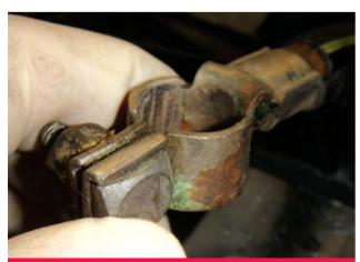
Remove the negative battery cable and wait three minutes before working near SRS components.
