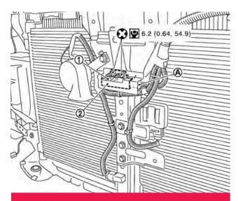
The Crash Zone Sensor is mounted in the front of the car so it's able to report head-on collisions before the shockwave can reach the occupants.
