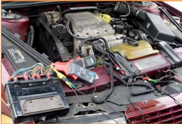
Figure 7: Installing 2 current probes at the ECM connector to check current at each injector bank
