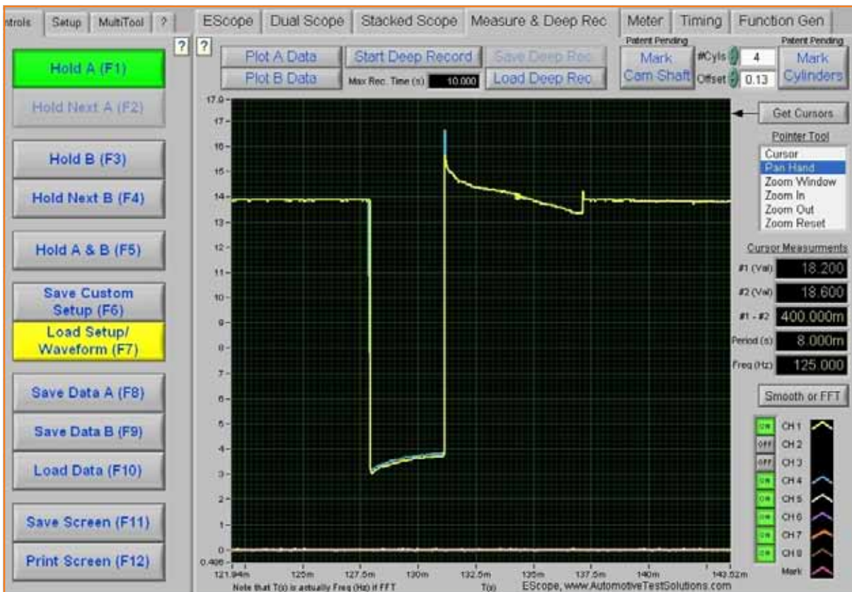
Figure 6: Scope checking the voltage trace of both injector banks
