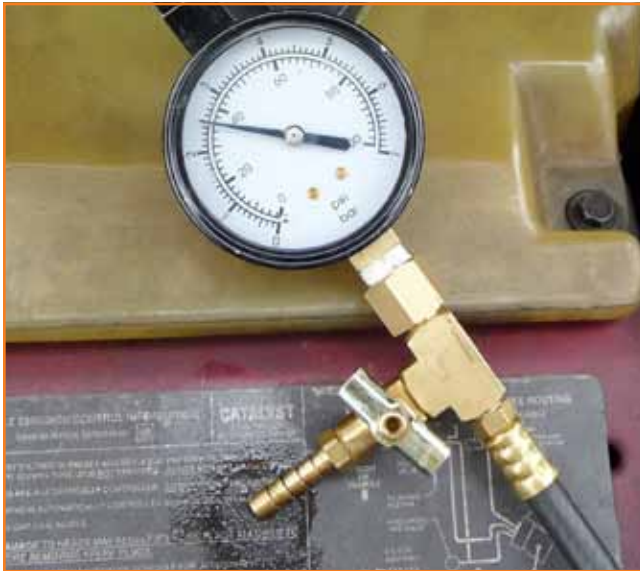
Figure 5: Checking fuel pressure with a gauge
