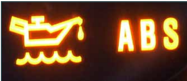
This is not the oil pressure indicator lamp! Instead of a maintenance required light, Subaru’s 2011 Outback has an oil level indicator.
