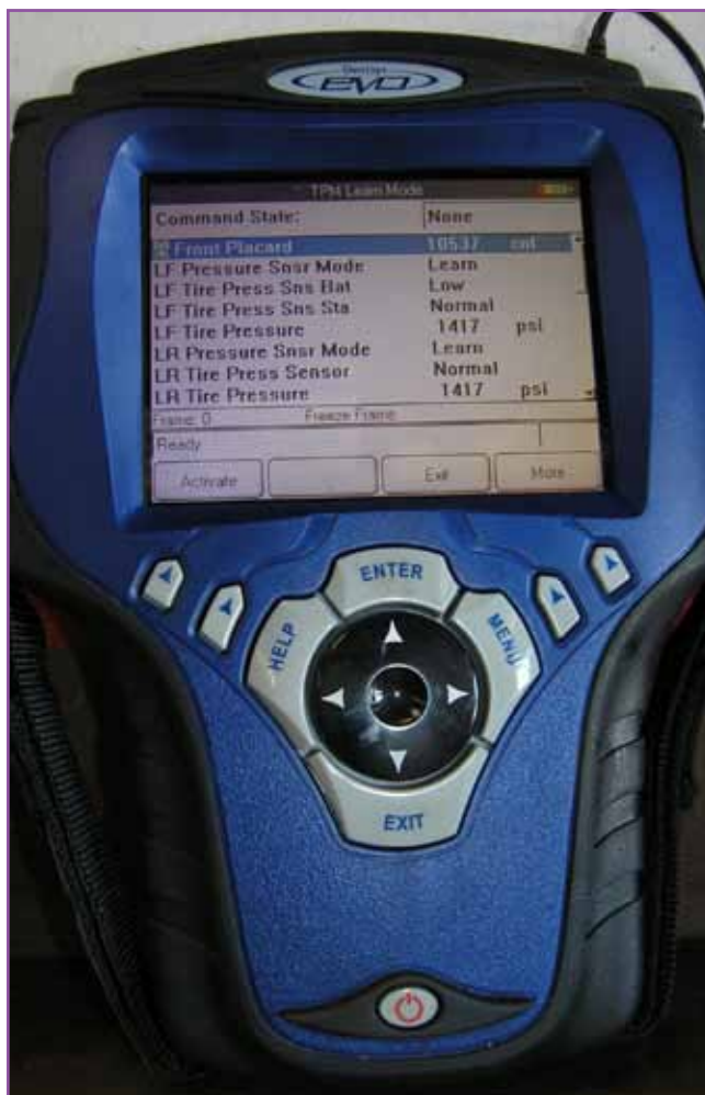
The TPMS tool function that is available for the Genisys can allow you to diagnose a vehicle with tire pressure monitoring system malfunctions.
