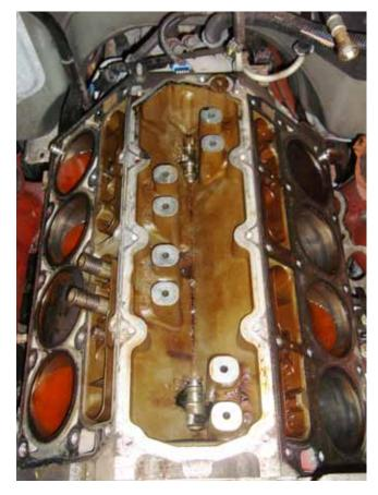
Left: The bosses sticking up from the lifter valley area are the passages that supply oil from the VLOM to each cylinder. Notice how they are only for cylinders #1, #4, #6 and #7. While you've got it apart, make sure the passages are clear.
