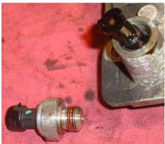
In the back of the VOLM, you'll see the oil pressure switch sticking up. Under it is a filter screen. Remove it and see if it is clogged. Lack of timely oil changes?
