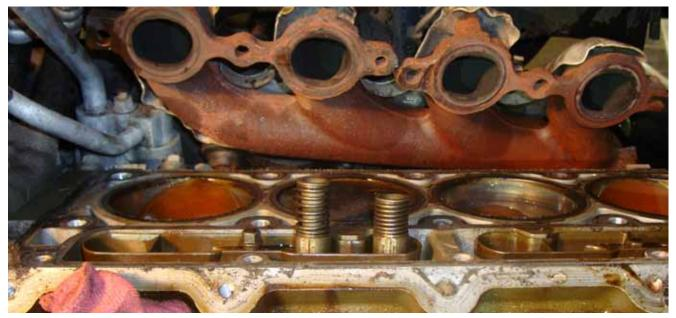
Here's the collapsed intake lifter for the #4 hole. This was a severe one with the lifter being completely stuck in the compressed position. The cylinder heads need to be removed to fix it.
