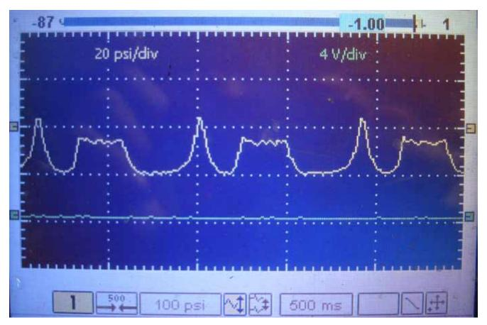
Below: If you have a pressure transducer, you can compare the misfiring cylinder to a good one and see if you have the same pattern. You should be able to determine if it is a sticking intake or exhaust lifter.
