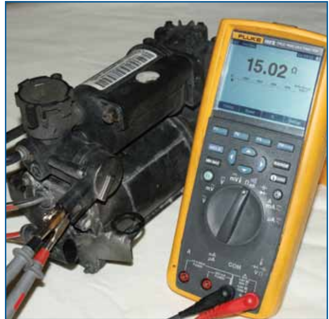
The heart of the Airmatic system is the air pump. It includes the pressure relief solenoid, which vents overall system pressure to lower the vehicle. If you have a case of no lift, verify that the solenoid is not stuck in the open position.
