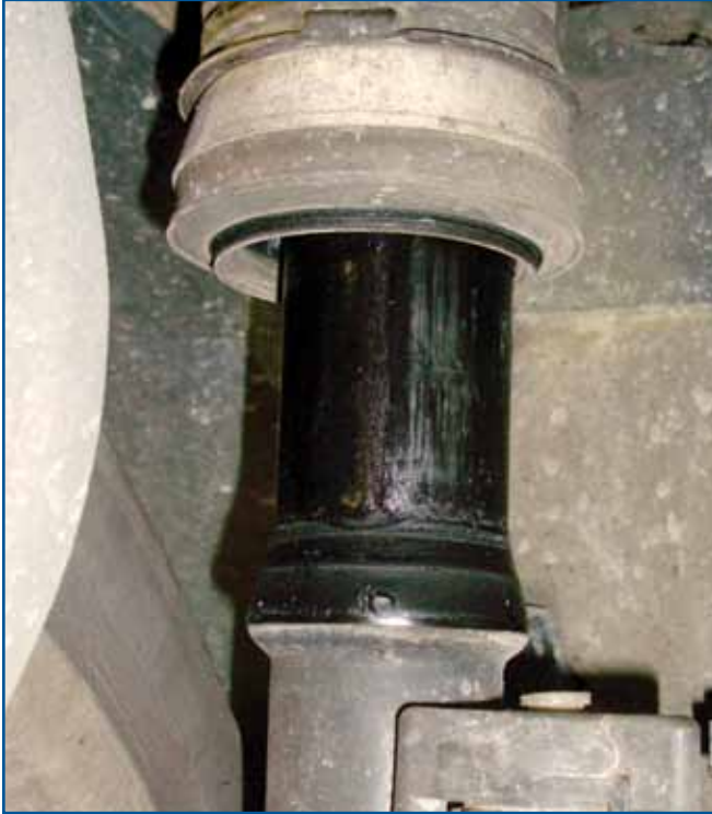
Here's a front shock assembly on a 220 chassis that has separated and allowed air to leak out of a system. This can happen from letting a leaking system go unrepaired for some time. You can also prematurely burn out the air pump from constantly trying to fill an empty system.
