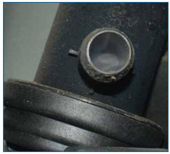
Here we are adding smoke and we have closed the cut-off solenoid. If you look closely, you can see a small amount of smoke coming from the vent. Is this enough to cause our leak code? We wanted to be sure.
