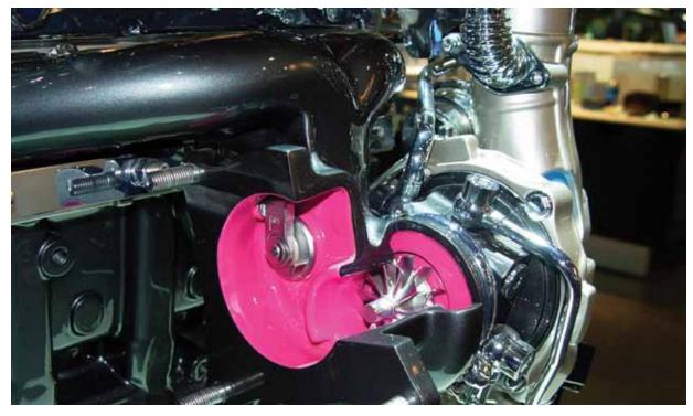
The exhaust exiting the engine spins the exhaust side of the turbo. If the boost pressure becomes excessive, the waste-gate shown here is forced open. This allows gasses to bypass the impeller and exit through the exhaust system.
