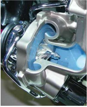
You are looking at the inlet side of the turbo assembly. The black valve at the bottom is the Recirculating or Divert Air valve. Under deceleration, this valve is commanded open by the PCM and any boost is redirected to the intake pipe of the turbo. The valve is closed again under acceleration.
