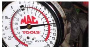
If you do not have a VAG 1397, you can use a pressure gauge but you are going to have to watch the gauge while someone else drives as the highest reading will obviously not be saved. Do this test in an isolated place.
