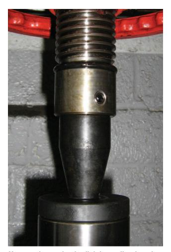
Use an adaptor that is slightly smaller than the outer race and does not contact the inner race to press the wheel bearing into the knuckle.
