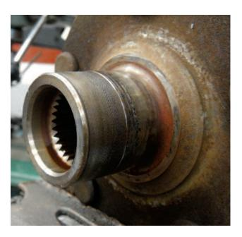
The most common problem is a seized bearing causing an inner race to spin on the hub. The race is a press fit, so if it's forced to turn, it will quickly start to gall and wear away at the hub.
