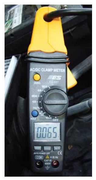
A low-current inductive pickup plugged into your meter can give you a ballpark figure of what kind of draw is present. Always back up your amp draw reading with a Volkswagen approved meter. You can find this and other service information at <u>www.vw.erwin.com</u>.
