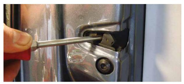
Make sure all of the latches are closed on any door, hood, or trunk that is open. The open door will keep accessories on longer and will give you a false amp draw reading.
