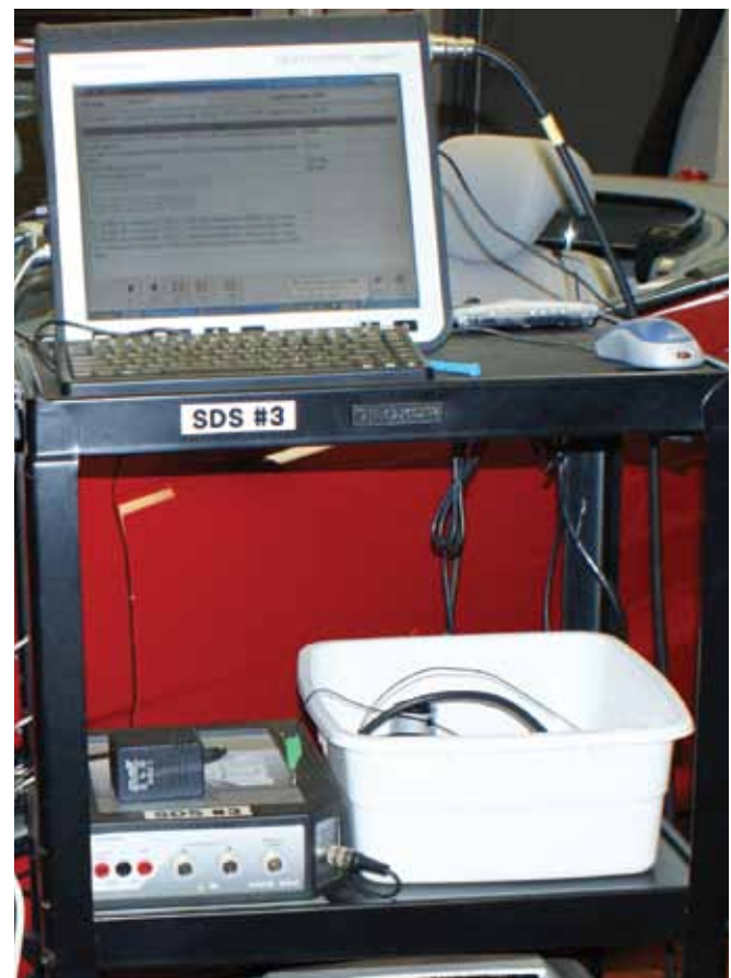
Above: Using your SDS, you can command a dynamic test (aka "Rodeo Mode") where the system applies and releases pressure to all four corners of the vehicle. Follow the on-screen instructions and accelerate the engine to 3,000 rpm so the pump can supply enough pressure for the test.
