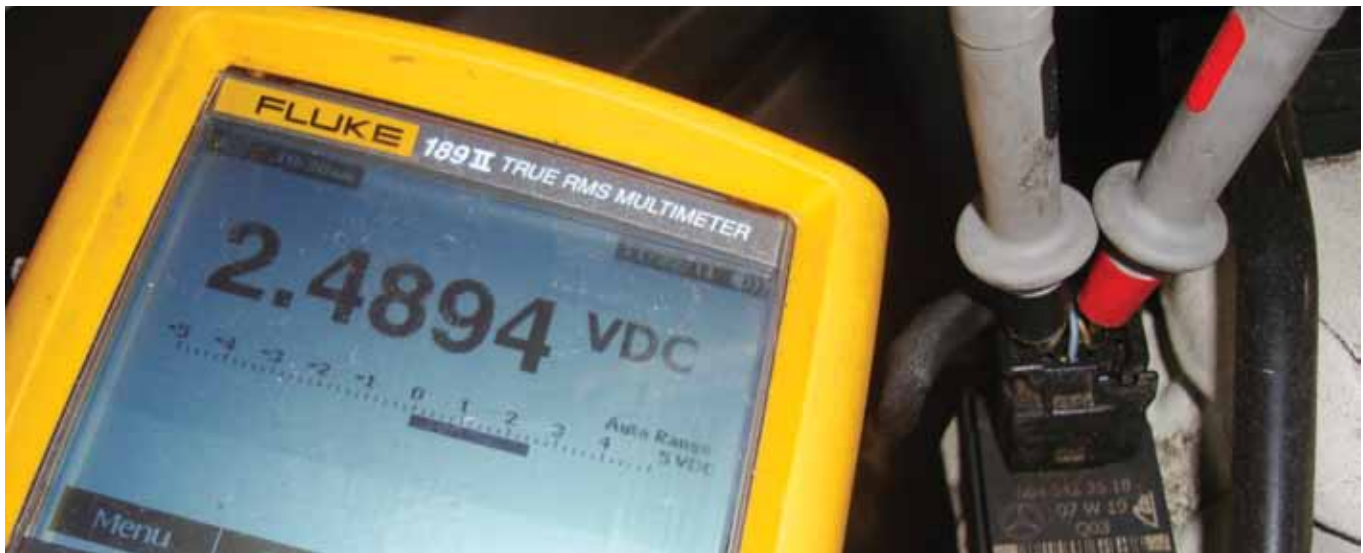
Above: In the static position on level ground the body acceleration sensors should read about 2.5V. As the vehicle moves, the signal voltage will increase or decrease depending on vehicle direction. If these sensors are off by more than a few tenths of a volt, the control unit will flag a code.
