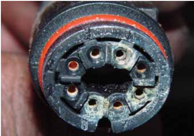
Take a close look at the EA harness connector. A problem here may be the cause of an intermittent throttle code and the customer complaining that the engine goes into limp-in mode. Corrosion at the pins can change the voltage signal enough to set a code.
