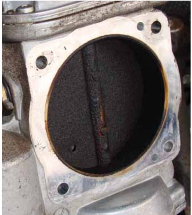
Carbon can build up on the throttle plate and in the bore. The ME control unit will adapt by opening the plate to maintain idle speed. If the battery goes dead, this adaptation is lost and the engine may not idle properly. After cleaning the throttle body, you may have a high idle, so clear all adaptive strategies.
