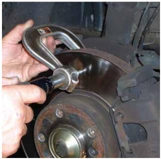
Even if they're not down to the discard thickness yet, how much iron was lost during the last wear cycle? If that same amount will take a used disc below the throw-away spec, you should have a talk with the customer about "rotor forecasting.
