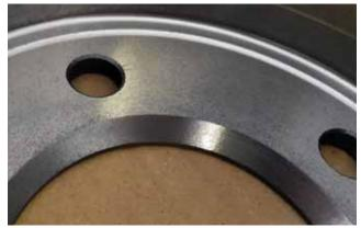
One subtlety most people don't know about is the angle of the chamfer of the center hub hole. Is it identical to O.E. on that aftermarket replacement?
