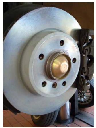
Perhaps you've been expending a lot of work cleaning that nice rust-preventative coating off a new rotor before putting it into service. You can stop now. It's meant to stay on and actually helps the bedding-in process to prevent squeaks and squeals.
