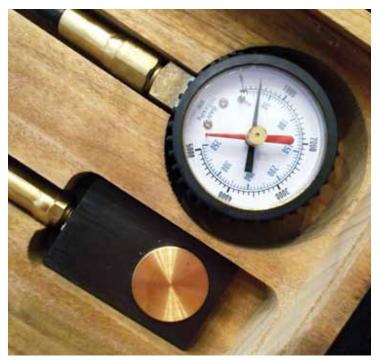
Is that brake pull being caused by a hydraulics issue, or did somebody do something strange like mixing brands of linings? Comparing the squeeze of each side will tell you.
