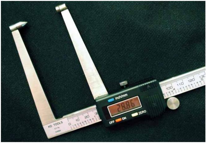
It may not be as accurate or rugged as a mechanical disc micrometer, but since our eyes aren't what they once were we've come to love our digital rotor caliper.
