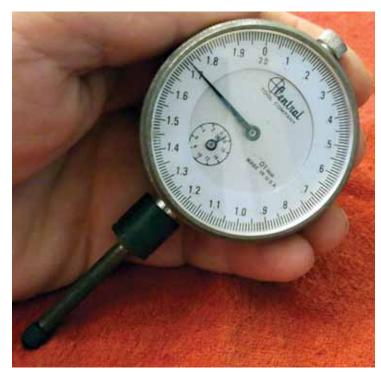
"Wobble" is commonly the underlying cause of DTV (Disc Thickness Variation), which in turn results in pedal pulsation. Use that dial indicator to head off comebacks.
