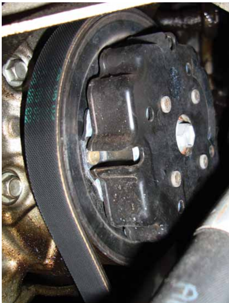
When you look at the pulley of a variable-displacement compressor, you'll see a rubber coupling instead of a clutch. A control valve in the rear of the compressor adjusts the output according to commands from the IHKA control unit.
