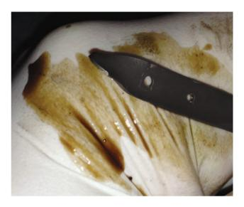
Transmission fluid becomes opaque and brown as it degrades. An acrid burnt odor and floating bits of clutch, bushing, and steel shavings are signs of trouble.
