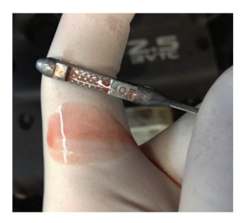
Transmission fluid should be translucent and free of floating debris. Most fluid is dyed red, but some fluids, like NS2, may have a different tint. Some types of fluid have a sweet odor when in good condition, but others can smell a little "sharp" even when new. Don't rely on odor as a gauge of condition unless you are familiar with what "normal" smells like.
