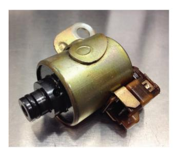
Solenoids can fail electrically (an open or short in the windings), or become stuck. Sticking is usually caused by fluid contamination. Fluid should be replaced if a stuck solenoid is found. However, if a transmission is worn and continues to dump debris into the fluid, a replacement solenoid may only be a short-term solution.
