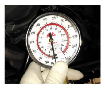
Fluid pressure does most of the work in the transmission. Use a pressure gauge to find out whether fluid pressure is adequate and if it's being directed properly.
