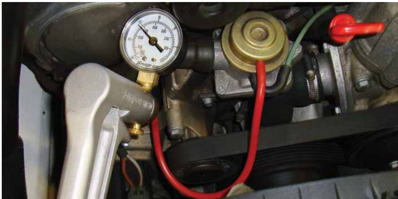
Here we are manually applying vacuum to the secondary air valve. The valve should hold vacuum. If not, the valve's diaphragm is torn and the valve needs to be replaced. You should activate the solenoid and verify vacuum is making it to the valve as well.
