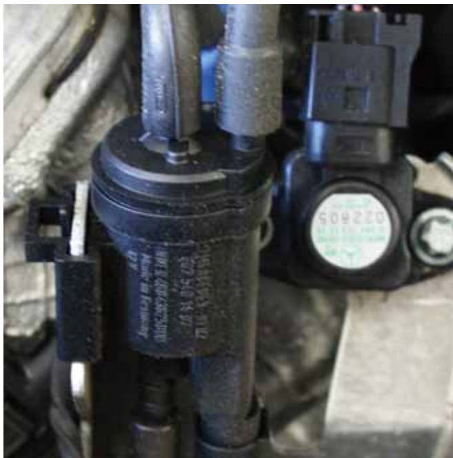
The air injection solenoid supplies the vacuum it gets from the intake manifold to the air injection valves. It is only energized when the engine is in the warm-up phase and when the monitor runs. If the solenoid malfunctions, the valves will not open and pumped air will not make it to the ports.
