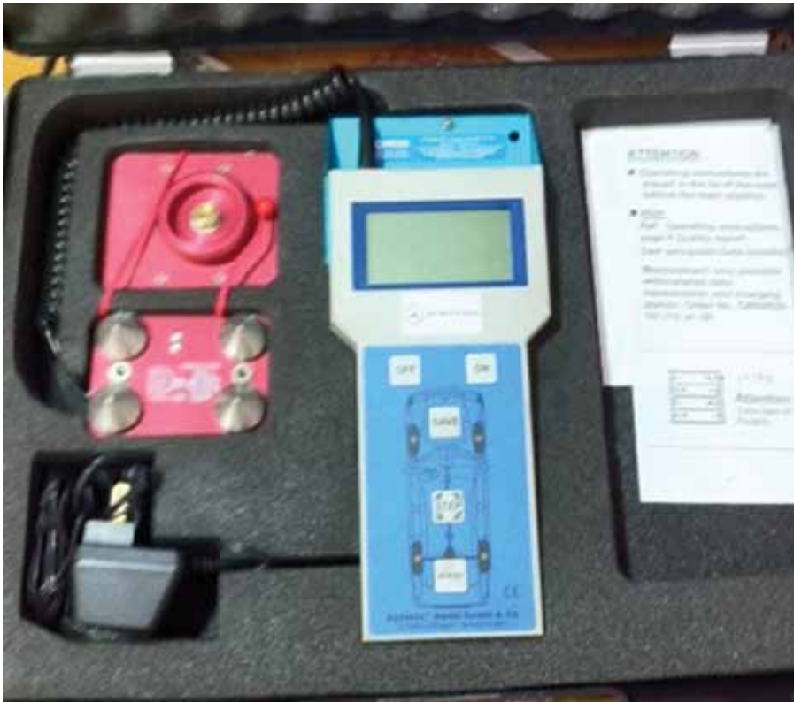
The Romess electronic inclinometer is a Mercedes-Benz-approved tool used to perform wheel alignments. (Image – Continental Imports)
