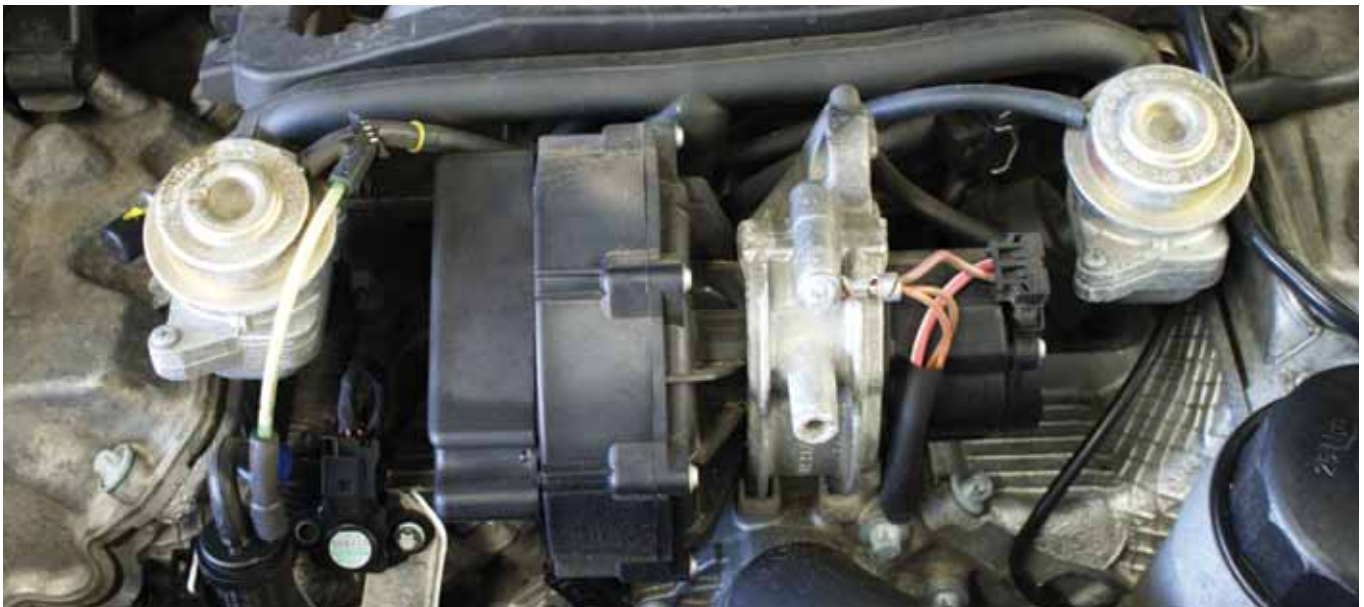
The modern secondary air pump on this 112/113 engine is mounted in front of the intake manifold so heat will evaporate any moisture that has condensed in the lines. It also makes manual testing easy. To the left of the pump is the air injection solenoid, and on the upper left and right are the air injection valves.
