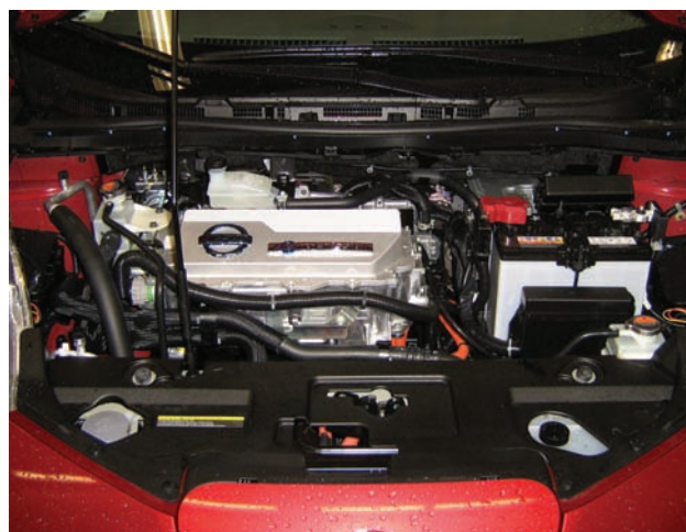
The stylish faux valve cover is set on top of the inverter unit and creates a traditional engine bay appearance.
