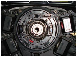
Not all inputs go directly to the EDC control unit. The steering angle sensor is built into the steering column module (SZL). The information is sent to the Gateway control unit and then passed on to the EDC through the PT-CAN.
